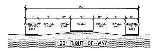
Figure 4. This figure shows an example of a typical 100-foot cross section consisting of four travel lanes, a raised median, and areas on each side for sidewalks, utilities, and street furniture. The outside travel lane has been allotted 17 feet to allow space for bicycle traffic next to the curb.
