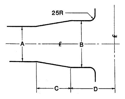
"A" equals mid-block width. The City Engineer will determine values B, C, and D when necessary for mid-block widths not in the following table (e.g., "A" equals 110).
