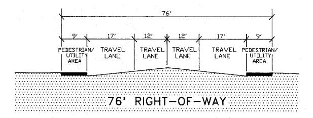
Figure 8. This four-lane version typifies the higher volume collector or the collector with significant truck traffic. Adequate space is provided in the outside lanes for bicycle traffic.
