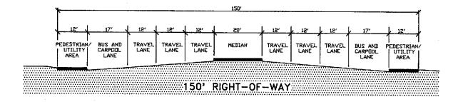
Figure 6. This figure shows how an exclusive bus, bicycle, and high occupancy vehicle lane could be included in a six-lane cross section. In this case, the sidewalk, utility, and street furniture areas are expanded to facilitate pedestrian traffic.
