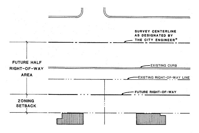
\*The survey centerline will be based on the section line or quarter section line along most streets.
