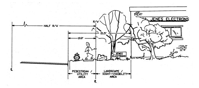
Figure 9. Typical cross-section between the curb and building on a 90-foot *MS&R* right-of-way street. This area contains provisions for pedestrians, utilities, drainage, landscaping, building setbacks and sight-visibility along both sides of the street. For details, refer to the *Tucson Zoning Code* and the City's *Development Standards*. Along *Major Streets and Routes* the building setback line is measured from the *MS&R* back of curb lines as required in the Zoning Code.
