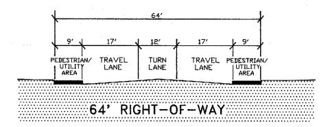
Figure 7. This three-lane example shows a standard collector street. The continuous turn lane allows the travel lanes to provide improved through traffic service. Adequate bicycling space is provided in each 17-foot travel lane.
