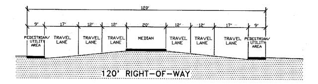
Figure 5. A typical high volume arterial cross section is shown in this figure, consisting of six travel lanes, a raised median with storage for turning vehicles and areas on each side for sidewalks, utilities, and street furniture. Seventeen feet has been allotted to the outside travel lane to allow adequate space for bicycle traffic next to the curb.
