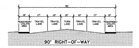
Figure 3. This figure shows an example of a typical 90-foot cross section consisting of four travel lanes, a continuous turn lane, and areas on each side for sidewalks, utilities, and street furniture, such as bus shelters. The outside travel lane has been allotted 17 feet to allow space for bicycle traffic next to the curb.
