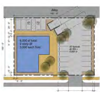
2 Story Building w/ Double Loaded Side & Alley Parking, Trash Enclosure and Alley Access 1" = 30'
