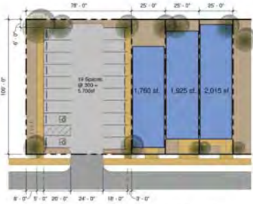
Double Loaded Parking Supporting Multiple Buildings 1" = 30'
