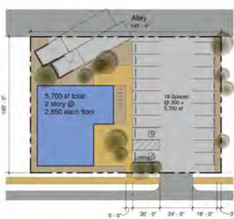
2 Story Building w/ Double Loaded Side Parking, Trash Enclosure and Alley Access 1" = 30'
