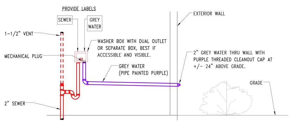
WASHER WALL BOX — SEWER NOT TO SCALE
