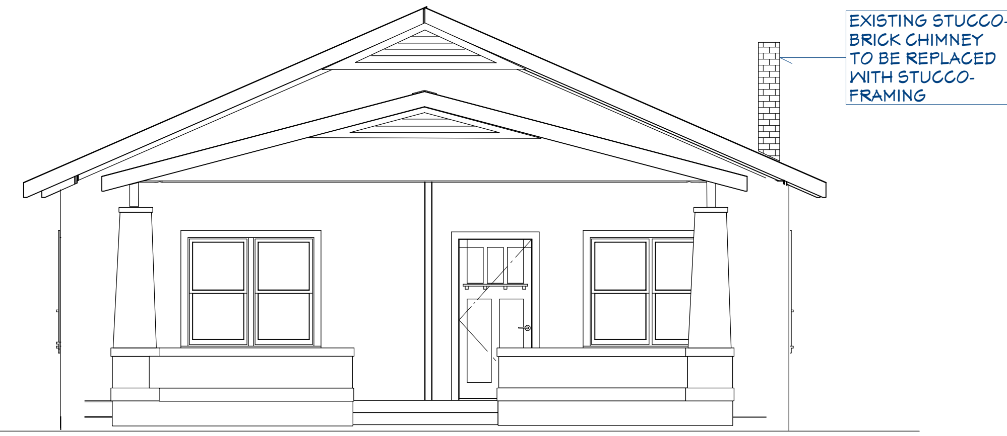
EXISTING EAST ELEVATION
