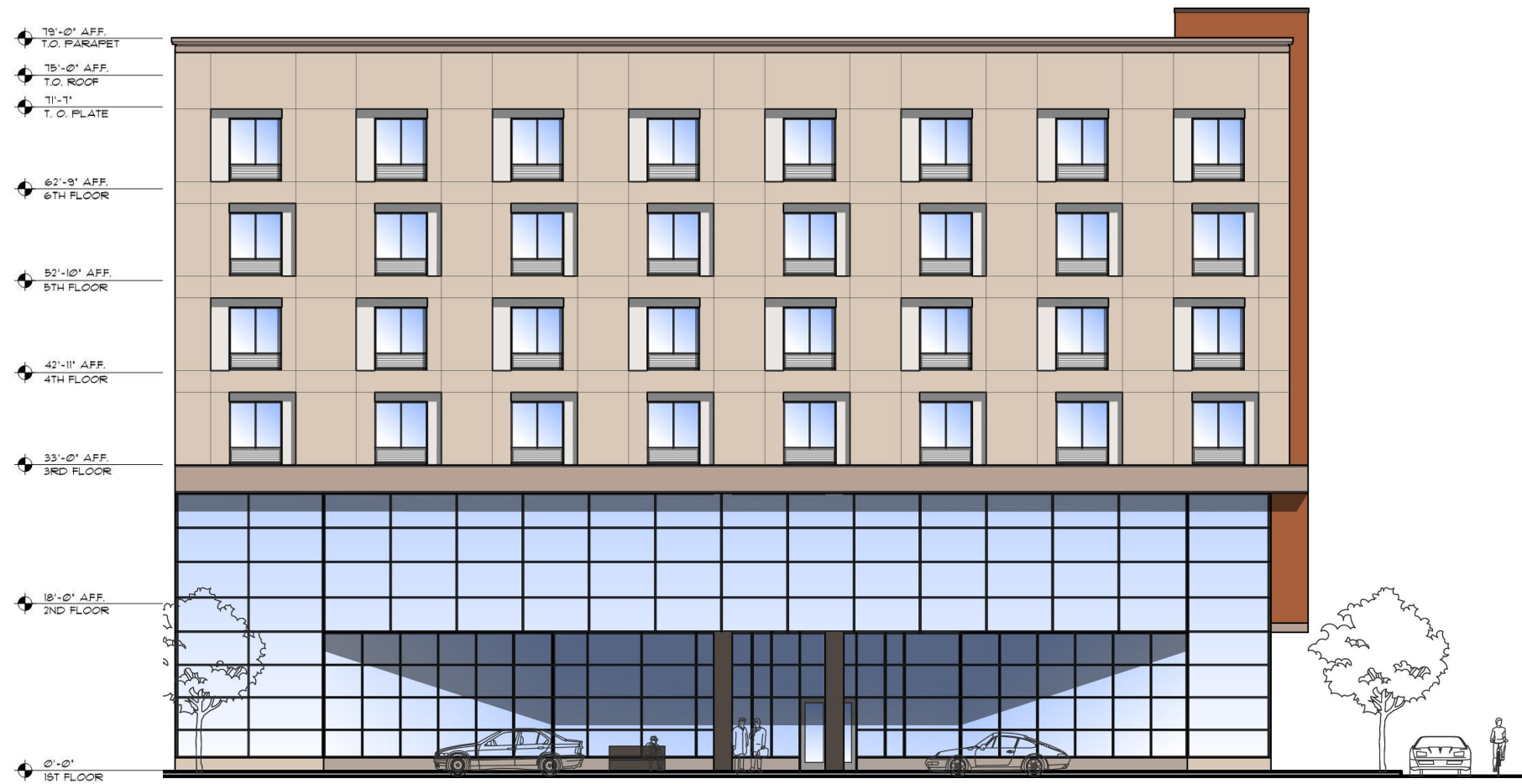
NORTH ELEVATION (FACING E. OCHOA ST.) SCALE: 1/20" = 1'-0"
