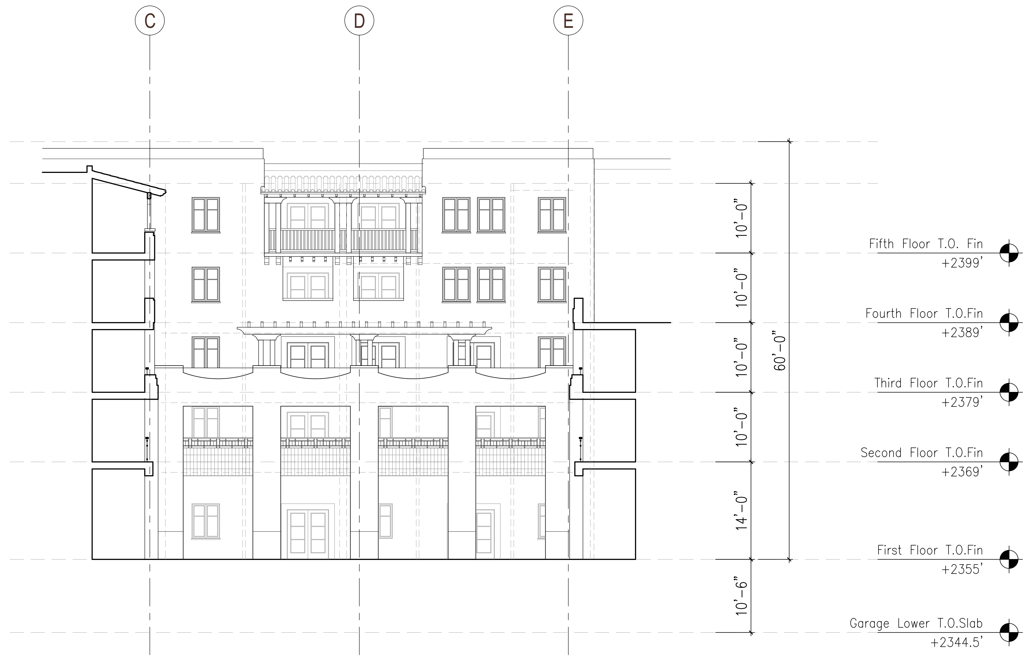
Courtyard D Elevation - West 1/8" = 1' - 0"
