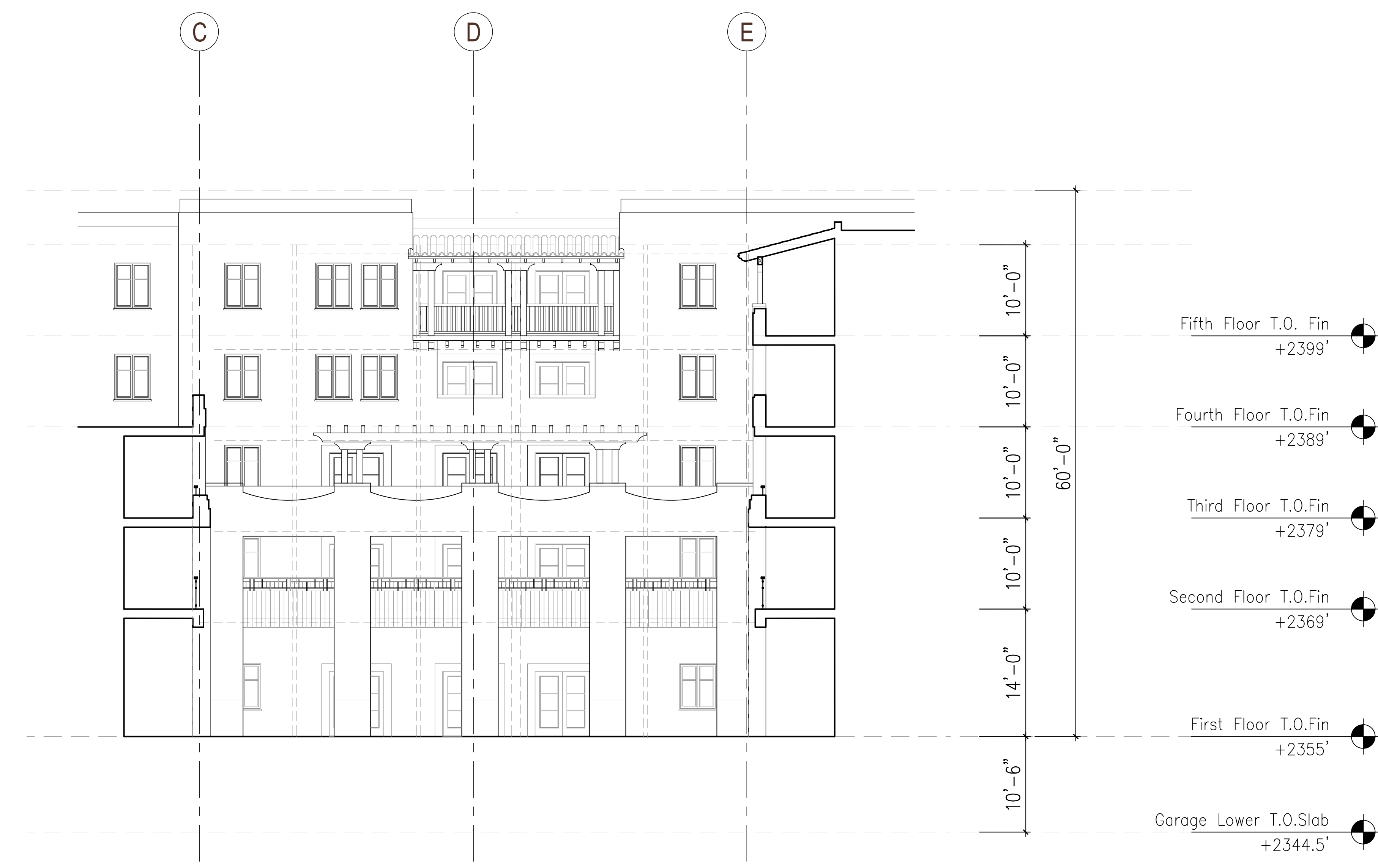
Courtyard C Elevation - West ① 1/8" = 1' - 0"
