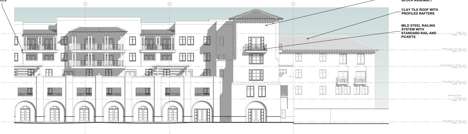
2 SOUTH ELEVATION - NORTH BUILDING SCALE: 1/8"=1'-0"
