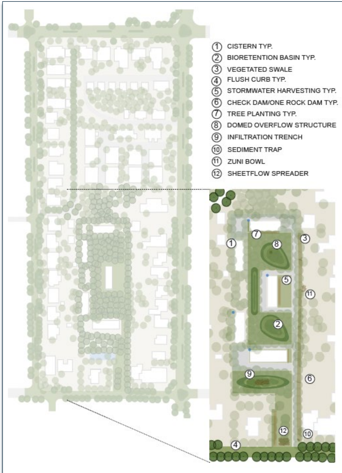
Figure 4.5. Zoomed in illustration of decentralized GI/LID infrastructure.
