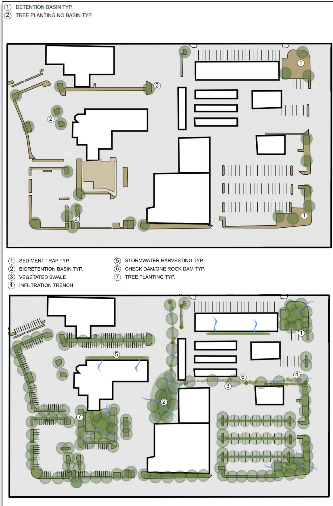
Figure 4.6. Centralized infrastructure and decentralized GSI for an example commercial development.
