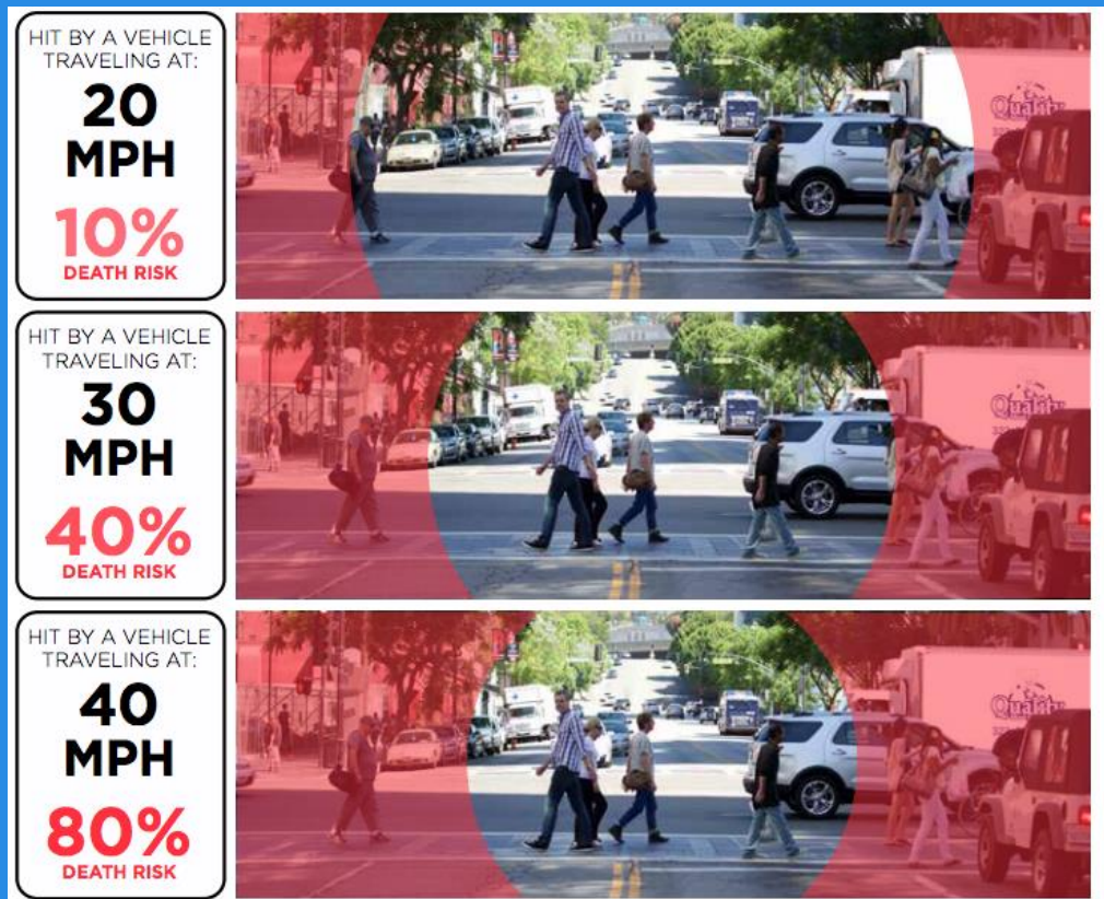
Figure 4. Impact of Vehicle Speed on Field of Vision and Risk of Pedestrian Death
