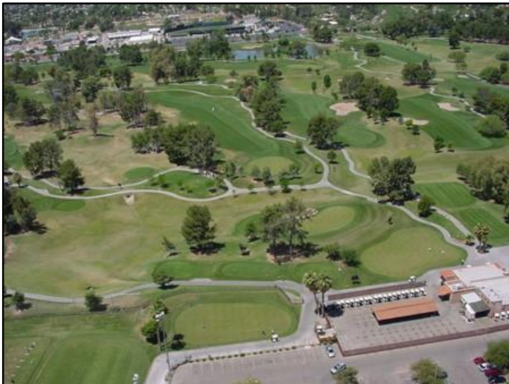
Figure 18: Phase I The fairways at Randolph South (like Kennedy Park) were reconstructed to be storm detention basins and are categorized as reservoirs.
