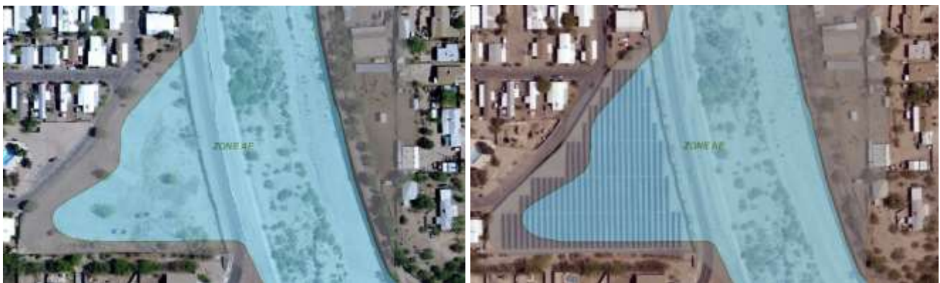
Figures 47 & 48: Before & after: dual purpose: ineffective flow area floodplain & solar project – reduces community’s electrical costs
