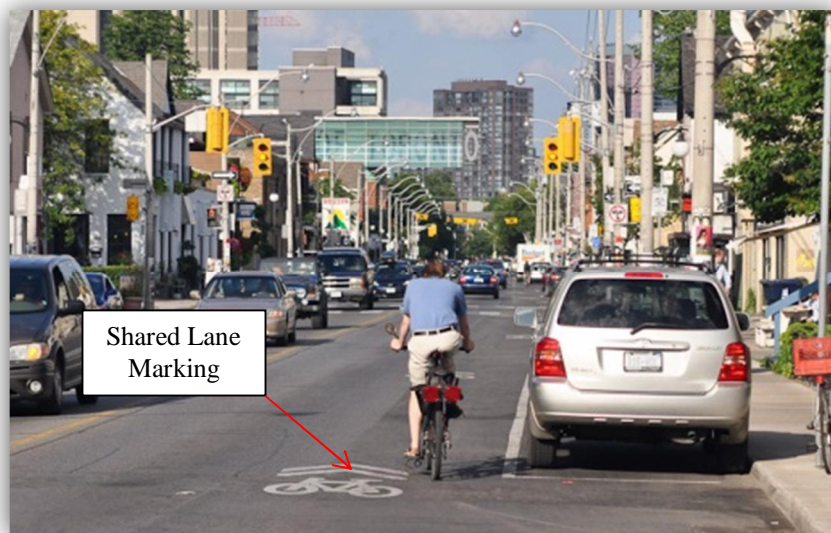
Figure 5 – Shared Lane Marking (Sharrow)
