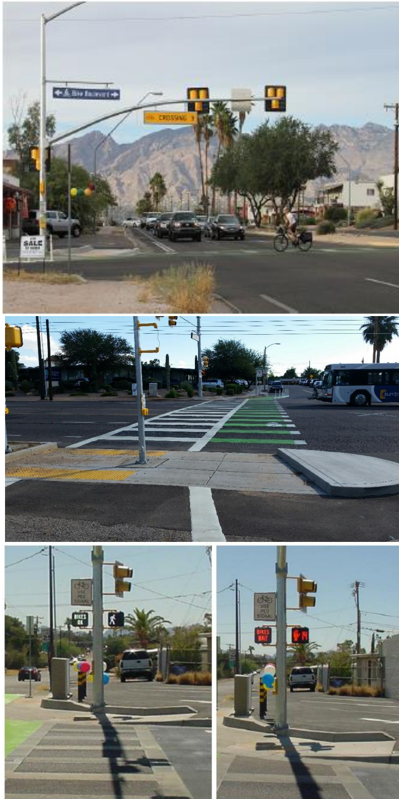
Figure 8: Examples of Bike HAWKs used in Tucson, AZ. 4
