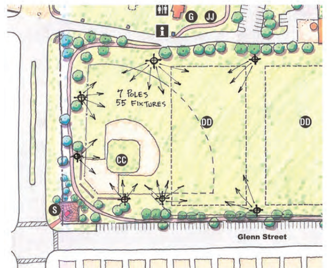
Figure 123: Proposed New Site Lighting for Baseball and Multi-use Soccer and Football Fields (DD).
