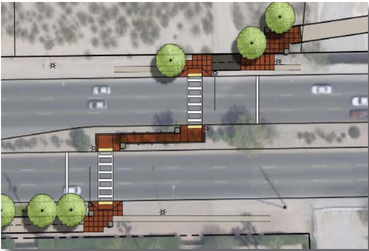
The layout of the Grant Rd. PELICAN crossing. This crossing suits the multiple lane and high volume nature of Grant Rd by providing users a respite area in the median of the crossing and halting one direction of traffic at a time, thus allowing for shorter stopping periods.
