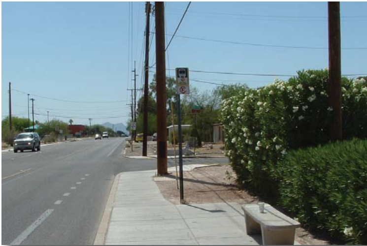
The right-of-way on the north side of East Glenn Street from Craycroft to W. V. Whitmore Elementary School is only about 11-feet wide with power poles in the center of the right-of-way, precluding the location of the multi-use path on the north side.
