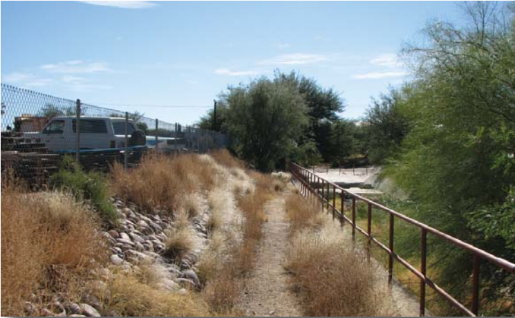
South of the city-owned parcel on Pima Street, the greenway path runs into a topographical challenge and vegetation existing that is desirable to save. The plan is to locate the path in a 15-foot area atop the topography using a retaining wall.
