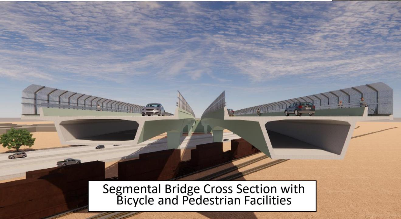
Segmental Bridge Cross Section with Bicycle and Pedestrian Facilities
