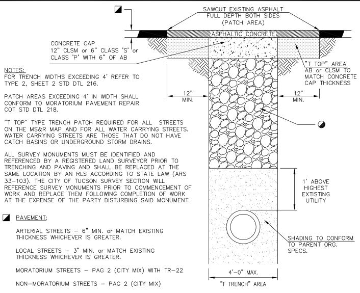
PAVEMENT SHALL BE SAW CUT, TACKED AND JOINED FOR THINNER SECTIONS
