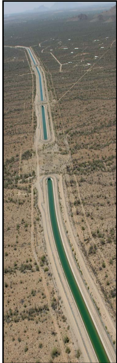
Central Arizona Project – This aqueduct brings Colorado River water from Lake Havasu to the Tucson area.
